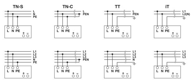
The connection for 100 V AC ... 240 V AC is established using the L, N, and P screw connections. The device can be connected to 1-phase AC networks or to two of the phase conductors of three-phase systems (TN, TT or IT systems in accordance with VDE 0100-300/IEC 60364-3) with nominal voltages of 100 V AC ... 240 V AC. The device also continues to work on short-term input voltages > 300 V AC.
